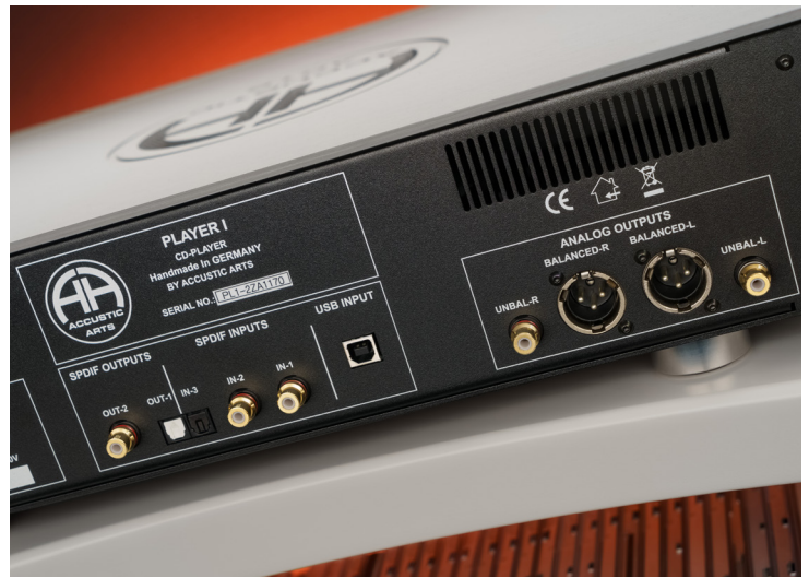
The "Player I" offers several connections. On the input side, it provides a USB port and three S/PDIF inputs. On the output side, it features balanced XLR and an unbalanced RCA connection in an analogue manner. You can attach digital devices via an electrical and an optical S/PDIF out.
